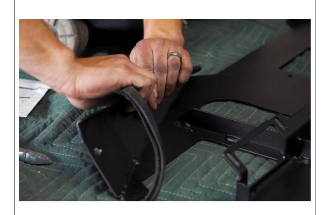
11. Fit pinch weld to top edge of main plate and wings.
